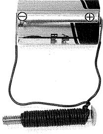
An electromagnet uses electricity to make magnetism. When electricity moves in a wire, it produces magnetism. If you coil a wire around a bolt many, many times, you make this effect much stronger. You turn on the electromagnet by sending electricity through the wire.
